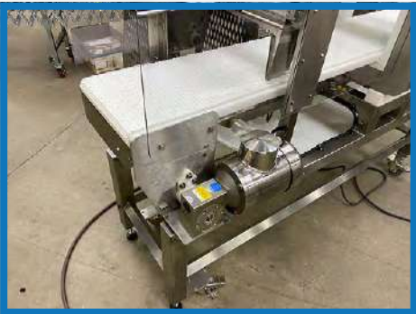
Stainless steel washdown gear-motor
