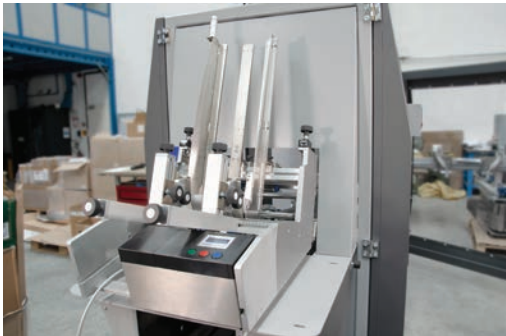
Large blanks storage, standard up to 1500 boxes. Expandable on request.
