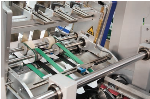
Blanks warehouse with precise release mechanism, precisely synchronised with the arriving product, equipped with a photocell indicating boxes almost finished.
