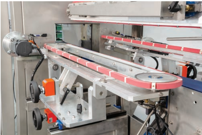
Output station with guide belts adjusted to the width of the box.
