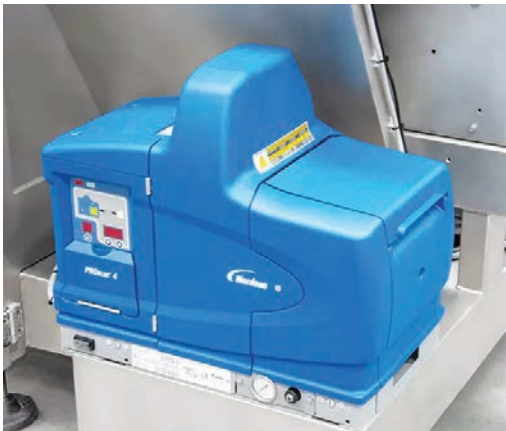
Hot met glue applicator to close the lower flaps by Meler, Nordson or Noxon, on the client's request.
